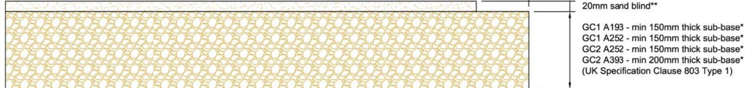
\*\* The sand blinding layer is intended to create a uniform seating for the Grasscrete formers and to prevent the loss of soil into the sub-base. It is not to be a regulating layer.
